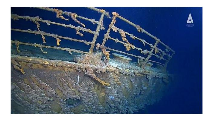
The footage from last year (a still is shown above) gives a much clearer look at the different parts of the ship that appeared in the movie. Titanic historian Park Stephenson said the deterioration is 'shocking', adding: 'That whole deck hole on that side is collapsing, taking with it the staterooms, and the deterioration is going to continue advancing
