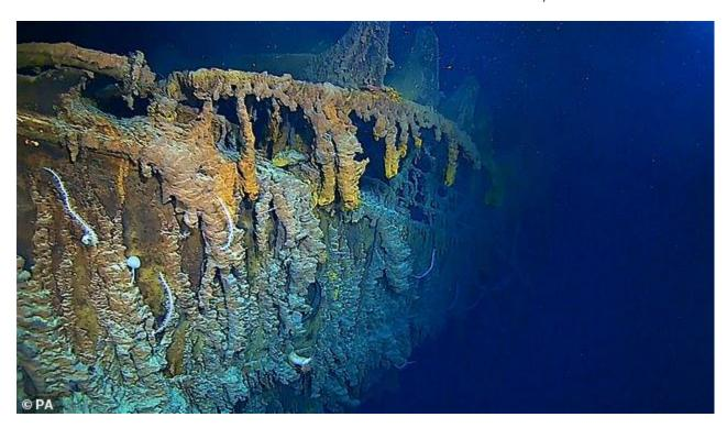
Around 13,000ft (4,000m) beneath the surface of the Atlantic Ocean, salt corrosion and metaleating bacteria have worn away parts of the liner's structure (pictured)
